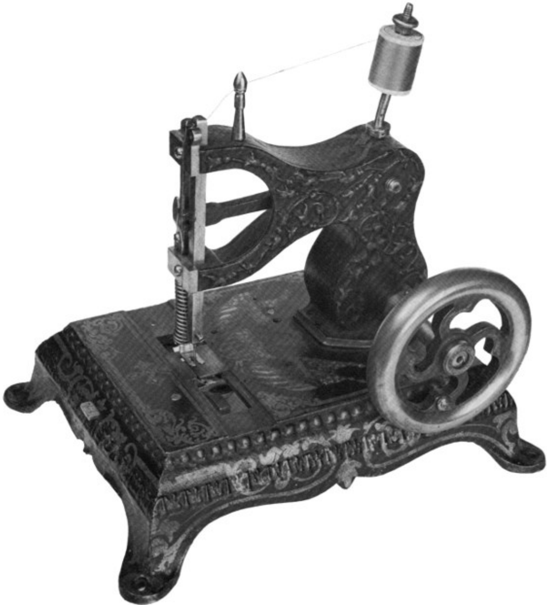
Figure 110.—NE PLUS ULTRA of about 1867. Another of the interesting hand-turned chainstitch machines of the late 1850s and
