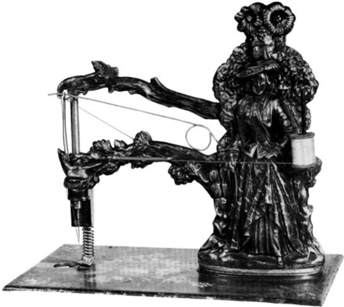
Figure 104.—“LADY” SEWING MACHINE of about 1859. The contemporary name of this machine is unknown. The unusual design of the head, or main support, is based in part on the design patent, number 216, of Isaac F. Baker, issued April 10, 1849, for a “new and useful design[,] for ornamenting furniture[,] called Cora Munro” who was a character in James Fenimore Cooper’s Last of the Mohicans . The design shows a female figure wearing a riding dress and hat that is ornamented with a plume and a bow. Her right hand holds a riding stick and the left, her skirt. Trunks of trees and foliage complete the Baker design, which is known to have been used for girandoles of the period. A companion design was also patented by Baker, number 215, which is in the form of a man in military costume and is named “Major Heyward,” for another character in Last of the Mohicans .
