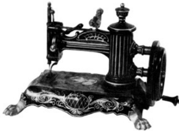
Figure 86.—EMPIRE SEWING MACHINE, late 1860s. Although an Empire Sewing Machine Co. existed in New York in the 1860s (the predecessor of the Remington-Empire Co.), it is not known whether this machine was manufactured by that same company, which was primarily concerned with producing shuttle machines. This chainstitch machine is marked “Empire Co., Patented April 23, 1863,” the date referring again to Ketchum’s patent. It is very similar to Folsom’s Globe, except that it has claw feet rather than a closed base; the painted designs on the base of both are almost identical to those on the Monitor. Its spool holder, mounted in reverse, is a crude imitation of the Folsom patent. The Empire machines were probably manufactured about the same time as the Wilson machine. (Photo courtesy of The Henry Ford Museum and Greenfield Village, Dearborn, Michigan.)
