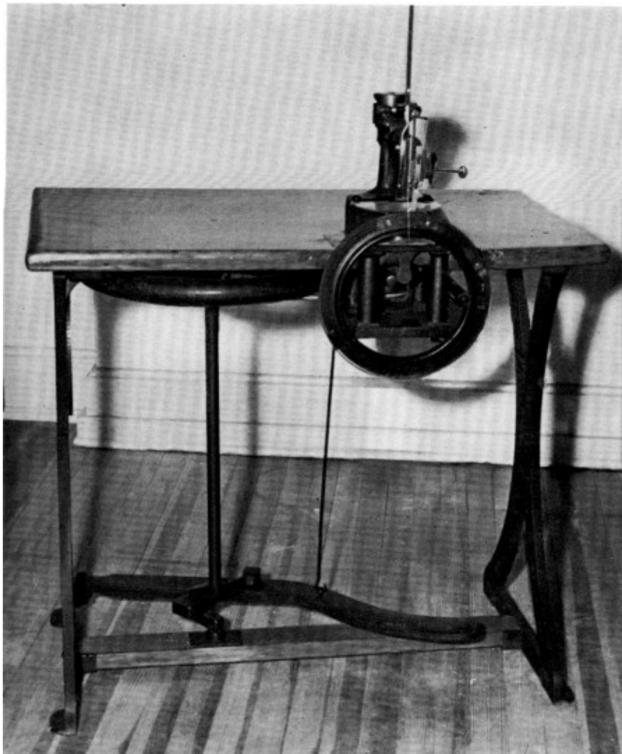
Figure 72.—A. BARTHOLF SEWING MACHINE, 1853. Abraham Bartholf of New York began manufacturing Blodgett & Lerow machines (see
