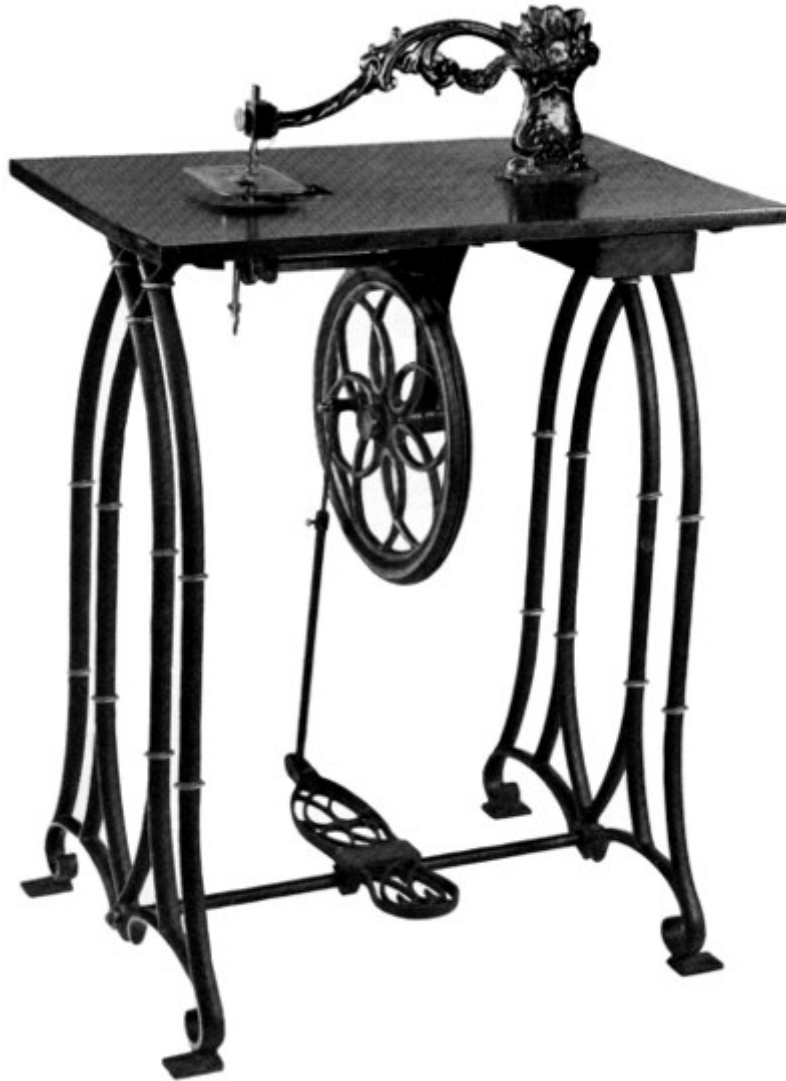
Figure 105.—LANDFEAR'S PATENT SEWING MACHINE of about 1857. Another of the many machines that, except for isolated examples, have almost completely disappeared from the records is Landfear's machine. Fortunately, this manufacturer marked his machine—where many did not—stamping it: "Landfear's patent-Dec r 1856, No. 262, W. H. Johnson's Patent Feb. 26th 1856, Manfrd by Parkers, Snow, Brooks & Co., West Meriden, Conn." (There was a Parker sewing machine manufactured by the Charles Parker Co. of Meriden, but his machine was a double-thread chainstitch machine and was licensed by the "Combination." The Landfear machine may have been an earlier attempt by a predecessor or closely related company.)
