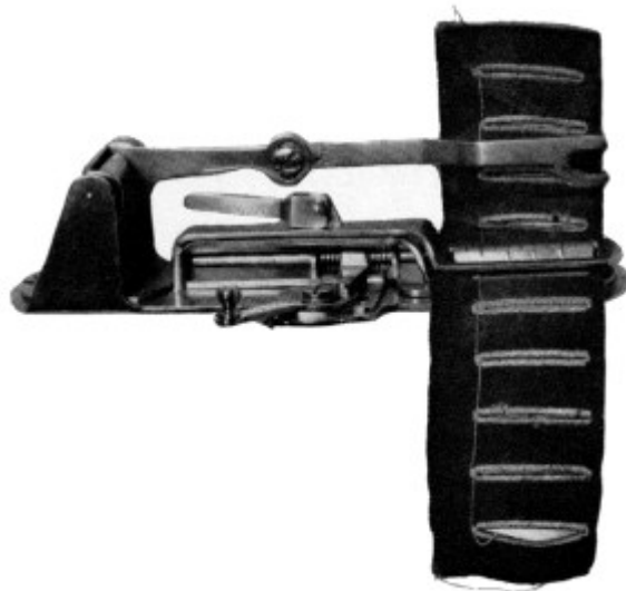
Figure 63.—HARRIS' patent buttonhole attachment, 1882. (Smithsonian photo P-63103.)
