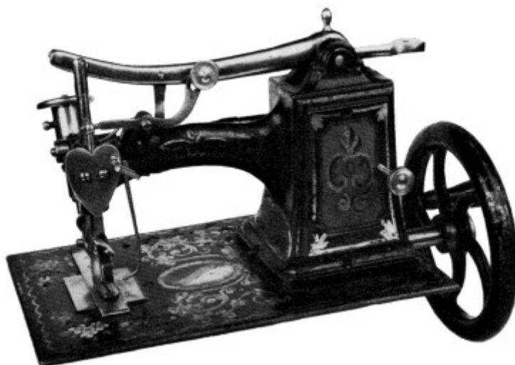
Figure 95.—[A.C.] HERRON'S PATENT SEWING MACHINE, 1858. The manufacturer of this machine is not known, but the machine was
