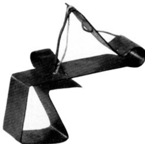
Figure 48.—HEYER’S POCKET SEWING MACHINE patent model, November 17, 1863. This patent model is one piece, and measures about two inches in height and two
