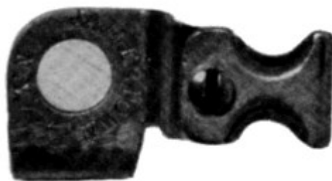
Figure 56.—HARRIS’ patent thread cutter, 1872. (Smithsonian photo P-6397.)
