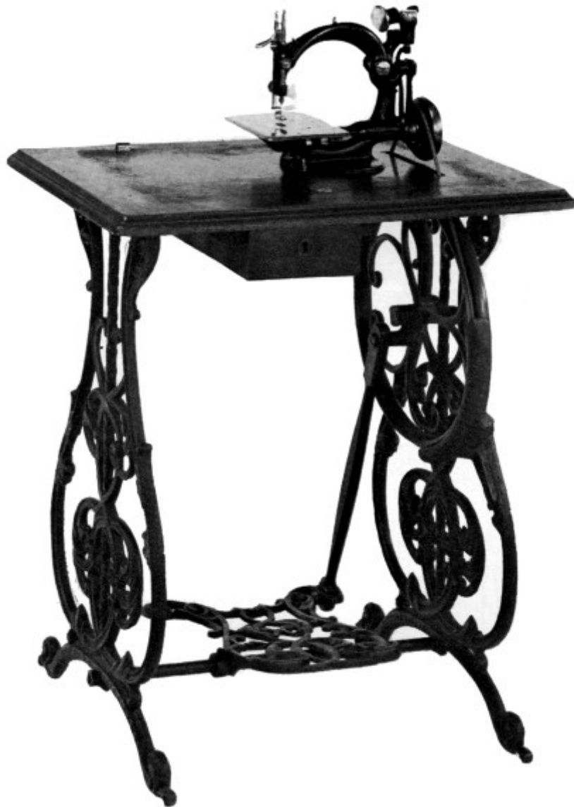
Figure 131.—WILLCOX AND GIBBS SEWING MACHINE, serial number 296572, of about 1878. From 1857 to the turn of the century, the style of the Willcox and Gibbs sewing machine changed very little (fig. 39). It was the most popular and the most reliable of the many chainstitch machines. In addition to the basic mechanical patents, Gibbs also patented the design of the sewing-machine head in 1860. In the specifications, he described it as an open ring set on a base or pedestal. The lower part of the open section supported the cloth plate. The design of the head, intentionally or not, formed a perfect letter G, the initial of the inventor. Later the machine head as a letter G was incorporated into the company's trademark. Additional
