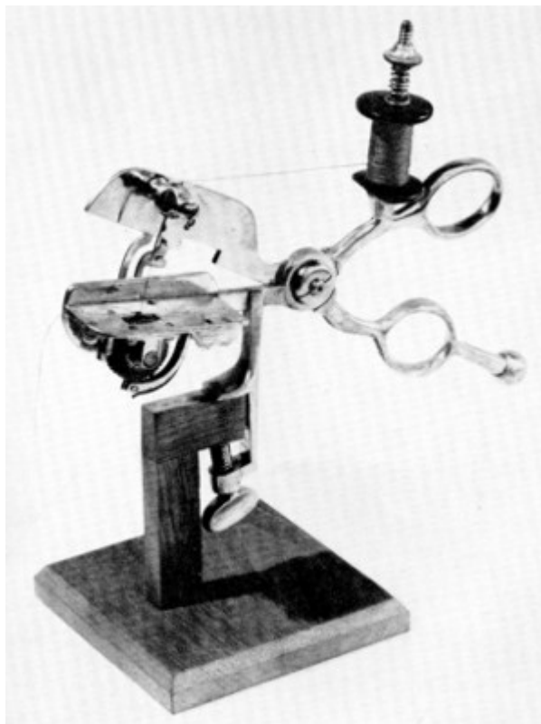
Figure 43.—THE SEWING SHEARS was another popular machine of unusual style. Some models were designed to both cut and sew, but most derived their names from the
