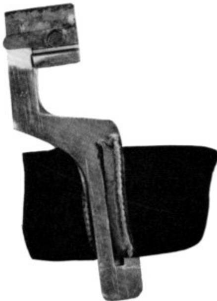
Figure 61.—SPOUL'S patent braid guide, 1871. (Smithsonian photo P-63102.)
